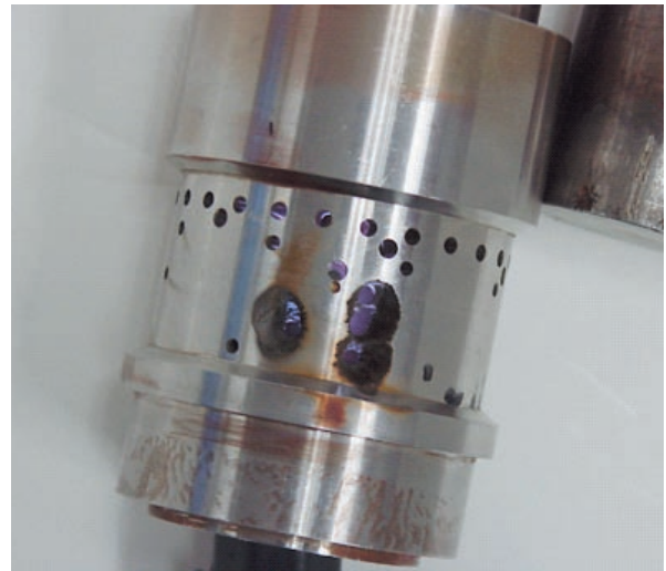
Figure 1: Cavitation and high velocity erosion of cage
