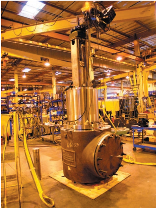
Figure 3: Complete valve undergoing shop test, section view of valve. Note all stainless steel construction.
