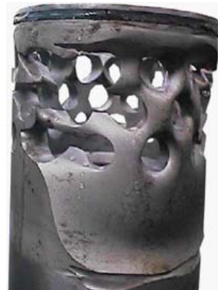
Single stage chokes have 1/5 the life expectancy of a 100DPC in severe service applications
